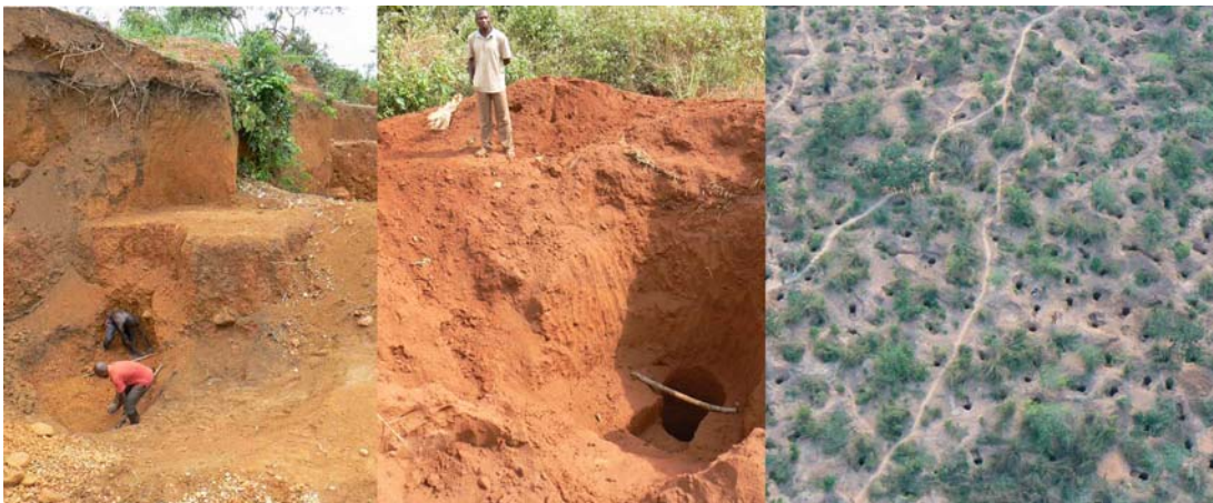
Figure 11. Left: creusers in an open quatre fois quatre pit (note the level separating the overburden of sand from the machanga gravel; middle: an active dijimba hole; right: part of an old chantier of thousands of majimba shafts.
