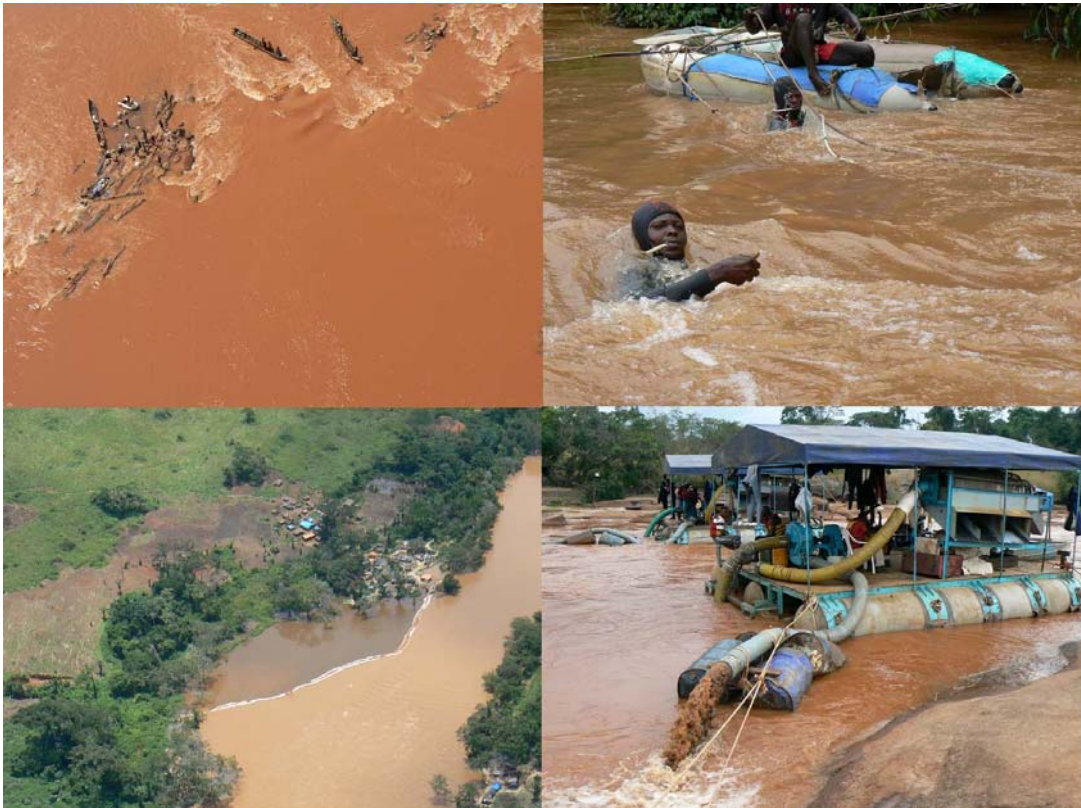
Figure 9. The four methods used for alluvial mining, clockwise from top left: diving off pirogues; divers with hoses from compressors; dredgers and a musapa created with sandbags.
